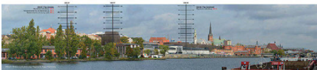
III. 8. Simulation of new buildings at Tobrucki Square, and Zawiszy and 3 Maja streets. VIS analysis height lines were placed at control points to show the scale of the development and its relation to historical components of the cityscape. By the authors.
