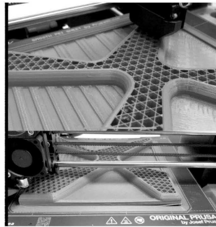
III. 5. A form used to fabricate architectural details - 3D printing. Author Wojciech Kocki.
