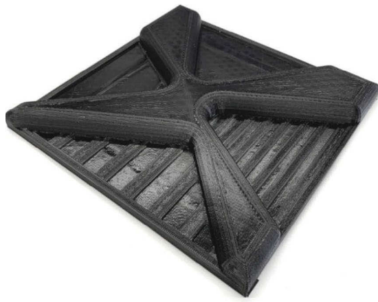
III. 5. A form used to fabricate architectural details - 3D printing. Author Wojciech Kocki.
