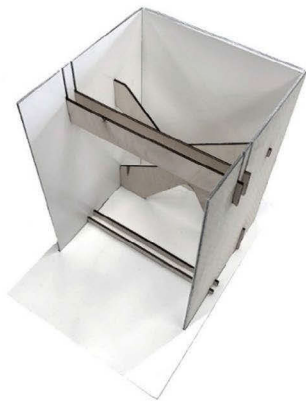
III. 6. The fabrication process of the remaining part of the casting module, laser CNC. Author Wojciech Kocki.
